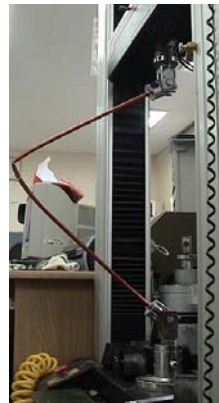
Acceptable tube breakage
