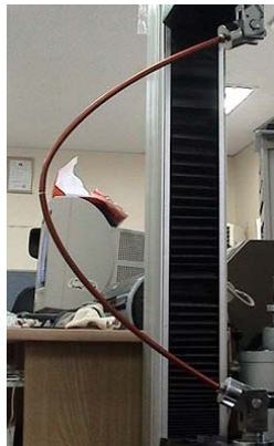
Acceptable tube breakage
