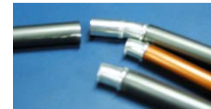
Unacceptable tube breakage (tube and FC split)
