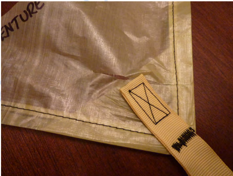
Figure 10 - Image of failed tieout after removal from test setup
