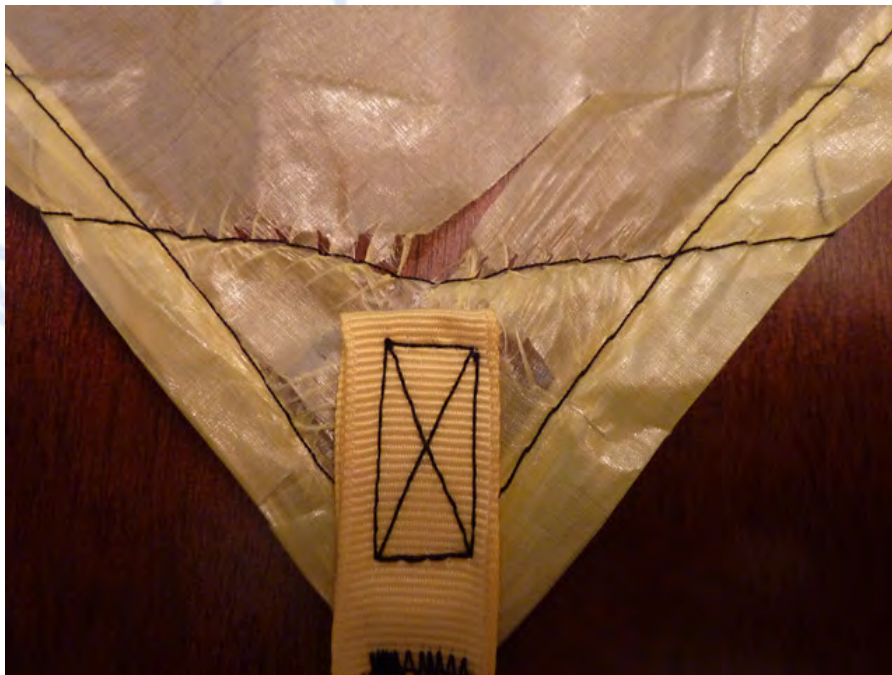
Figure 4 - Image of failed tieout after removal from test setup
