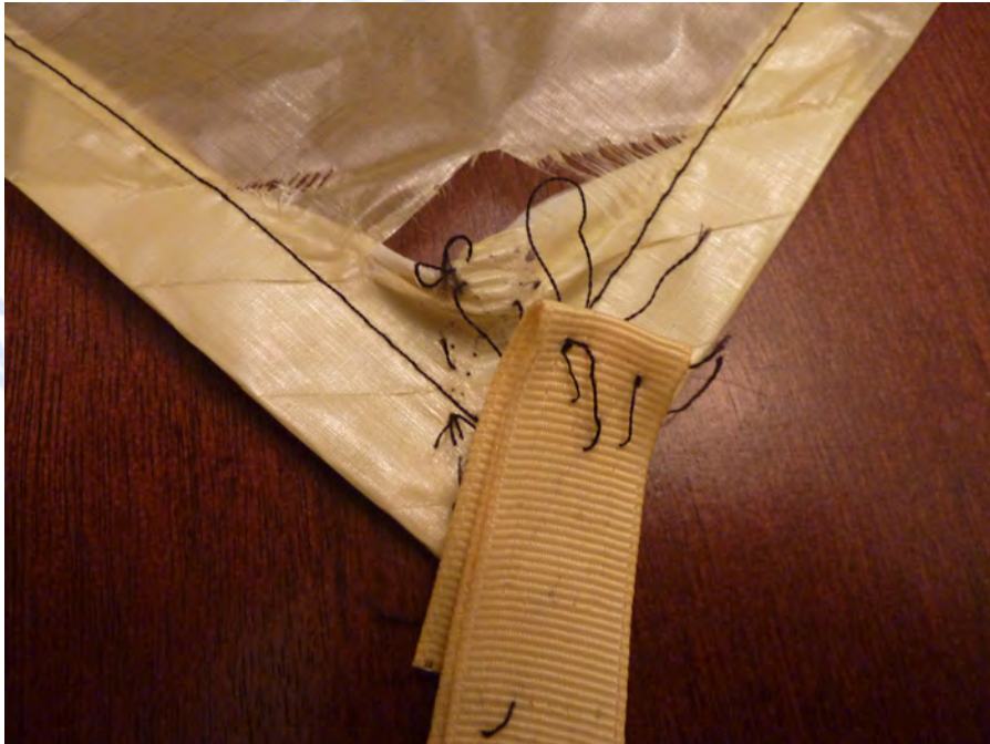
Figure 12 - Image of failed tieout after removal from test setup
