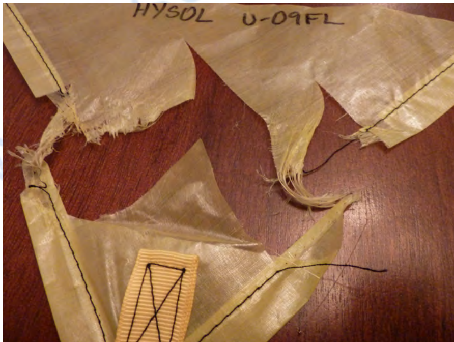
Figure 8 - Image of failed tieout after removal from test setup
