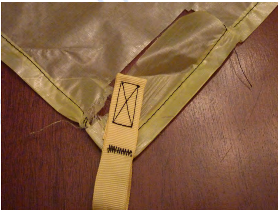
Figure 6 - Image of failed tieout after removal from test setup
